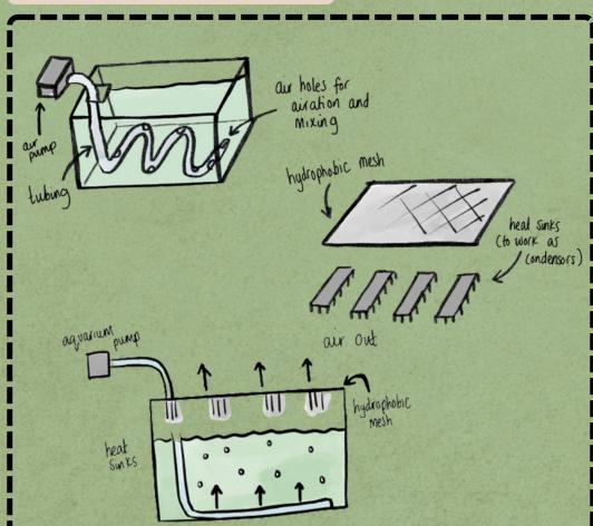
The algae needs a constant supply of outside air, this could have been done by simply keeping the lid open but we decided to optimise this process by using an air filtration system to maximise the surface area of the algae that is exposed to CO2. This results in our photobioreactor being incredibly efficient though we are compromising on energy usage as it will require more to power the pump.
